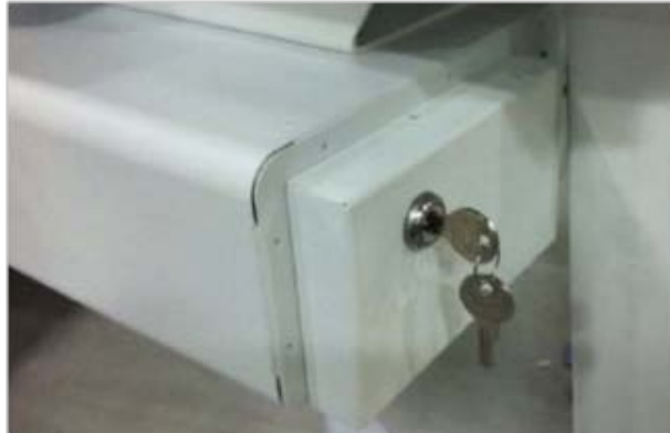
Rescue key access on back of drawer/cabinet assembly
