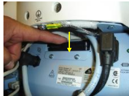
Press down to close filter cover
