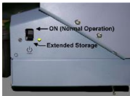
Flo MPE-7800 NiMH Power Supply “ON/Extended Storage” Switch
