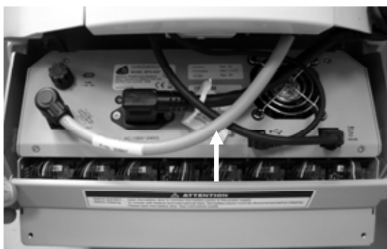
Rotate the Battery Connector Access Panel up to close
