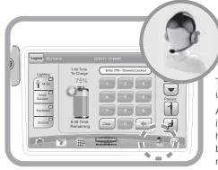
The **Service Request** button is used to send requests from the cart.
