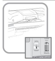
Task lighting is included to enhance cart usability in darkened patient areas. All CareLink carts are equipped with a standard keyboard light operated by using the **Lighting** button located at the left side of the touch screen.
