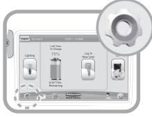
The cog button located at the bottom left of the touchscreen is used to access both the **Settings** and **Preferences** screens. If no user is logged in, the cog button will access the **Settings** screen. When a user is logged in, the cog button will access the **Preferences** screen.
